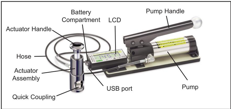
The *PosiTest AT* powers-up and displays dashes when the
