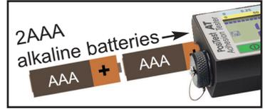
*USE ONLY AAA ALKALINE BATTERIES.* Nickel-cadmium and nickel-metal hydride rechargeable batteries will work but the low battery symbol may stay on.
